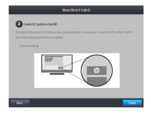
A confirmation window will appear, instructing you to complete the substrate creation process by making an ICC profile in the RIP.
